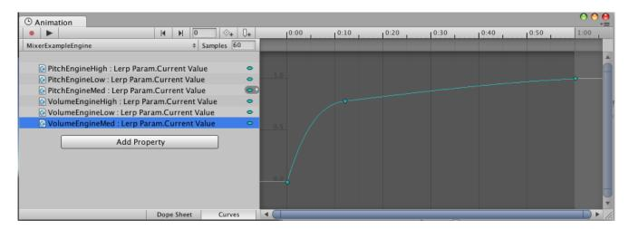
The left side of the curve will be the value when the ParamAnimation paramValue is set to 0 and the right side of the curve will be the value when paramValue is set to 1. Changing the paramValue will sample the LerpParam curves anywhere between 0 and 1 seconds.
